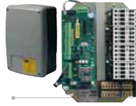
ABKS162 KS2/R4 control board for 2 3-PHASE SUPER 6000 with box
