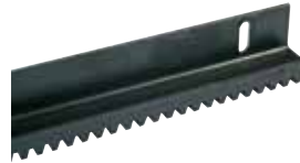
ACS9040 Module 4 RACK in iron (sect. 22 x 22 mm) with right-angle member (up to 2200 kg) in 2 m bars per m
