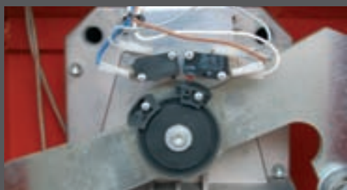
Perfect movements thanks to three limit switches.
