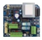
Suitable for these 230V operators: K5 - K500 - K800 - K800 FAST - K1400 - K2200
