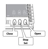
The programmable functions available are divided into 2 levels and their relative operating status is displayed by means of the 8 LEDs (L1...L8) on the control unit (LED lit = function active; LED off = function not active).
