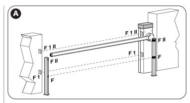
It is possible to install the TX or RX photocell inside the caisson of the barrier, in the space provided (fig. 43).
