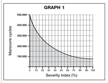
Example of calculating lifetime of road barrier S-BAR (refer to Table 2 and Graph 1):
